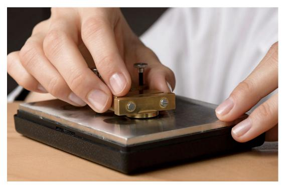
The surface of the stop click cover is flat-polished on a tin plate (top), and a specially shaped grinding peg is used to sharpen the reentrant angles of the tourbillon cock cover (right)
