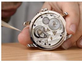
During the final assembly process, the watch is endowed with its fine face and cased up
